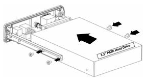
4 Place the hard drive with the plastic cap back into the aluminum housing and secure it with the two screws you previously removed.
